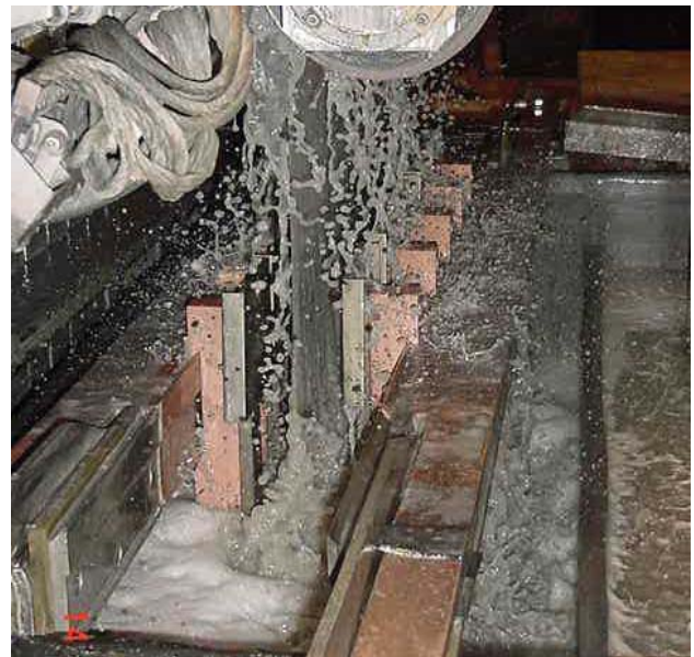
Figure 4 - Insoluble anodes in industrial plant
