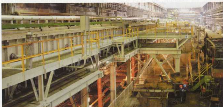
Figure 1. Pickling line No.1 was modernized to reach a nominal capacity of up to 2,200,000 t/year
