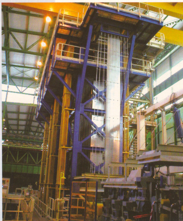
Figure 2. Looper of the tinning line at ArcelorMittal, Spain
