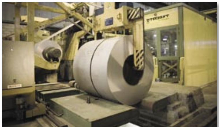
▶ Figs 1-2 The hybrid push-pull and semi-continuous pickling line at Duferco la Louvière
