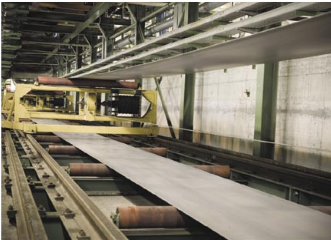
📌 Fig 3 The hybrid push-pull and semi-continuous pickling line at Duferco la Louvière
