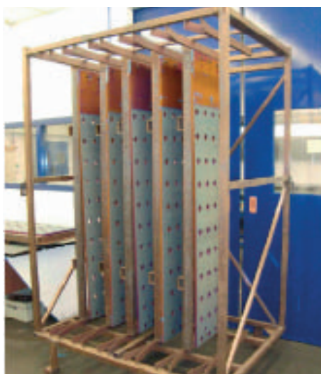
Fig 6 Insoluble anodes in the rack during MMO coating
