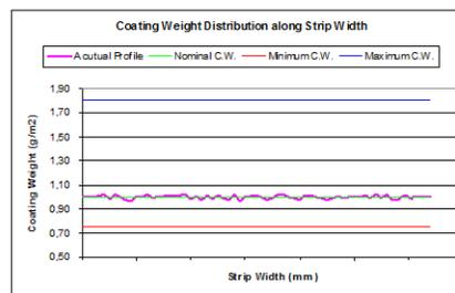
The solution to these problems is to equip the tinning line with insoluble anodes. They have a continuous surface and therefore very thin tin coating layers can be produced with high thickness homogeneity.
