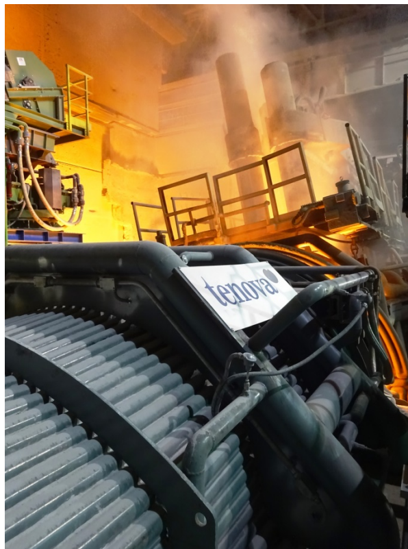
Fig. 7 – The new revamped Consteel® in operation, tapping phase.
