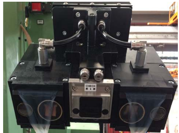
Figure 4: Inspektor 3 with EC, UT and CW probes
