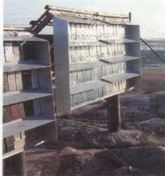
2 Vertical north facing 'under eaves' testing at Bohus Malmö is a more severe natural test
