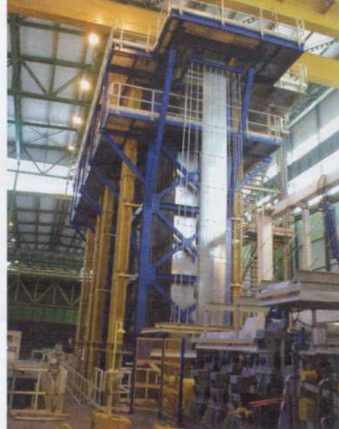
1 The new 250kt/y tinning line at Aceralia Aviles
