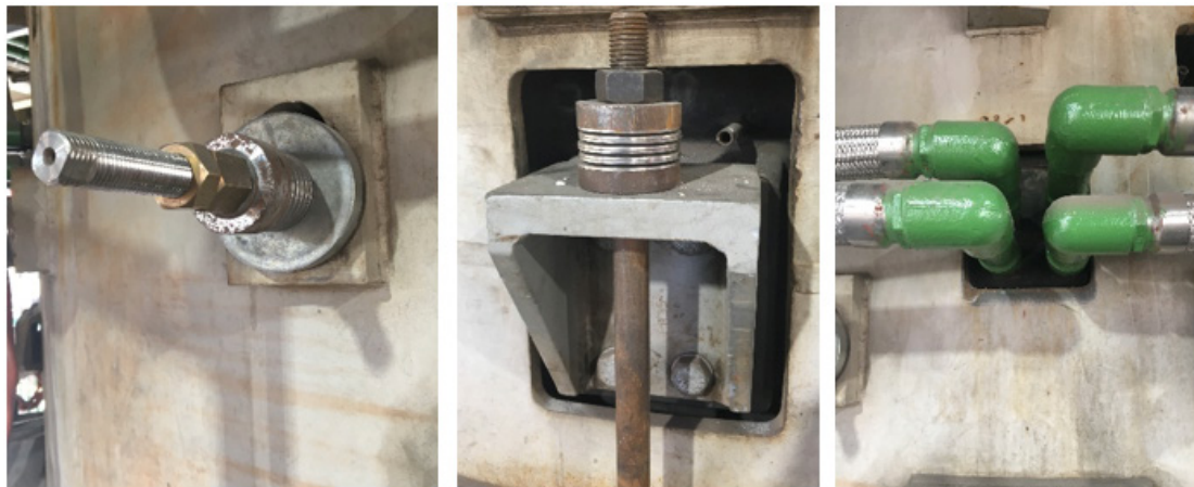
Figure 4: MAXICOOL® cooler shell connection, hold down mechanism and cooling water connections.
