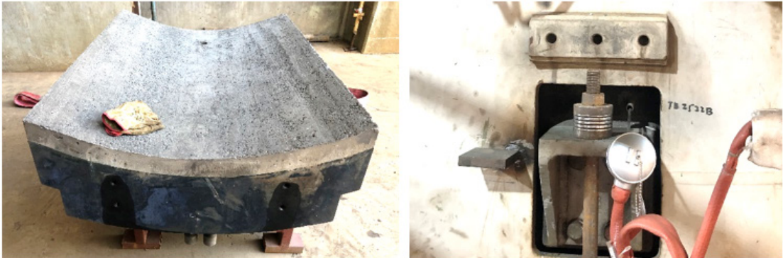
Figure 5: MAXICOOL® cooler with sacrificial refractory layer and typical copper thermocouple installation
