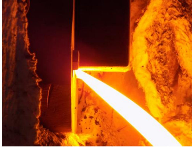
Figure 6. SlagFlo™ device in operation – tapping rate being reduced
