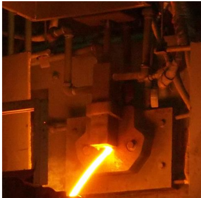
Figure 7. Installed SlagFlo™ device in operation
