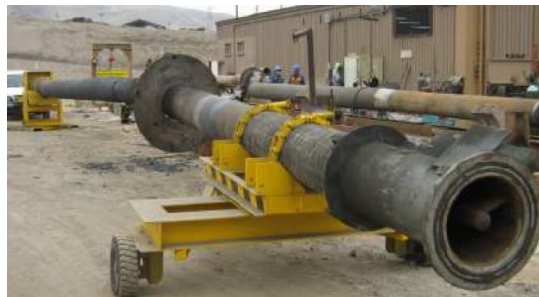
Figure 2. Severely bent TSL furnace lance being transported to the workshop for repair (Zambrano, 2010)
