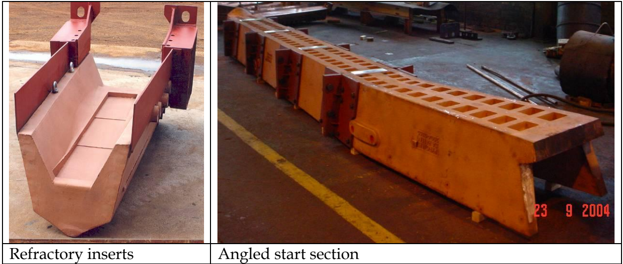
Figure 3: Examples of customised profiles, shapes, and lengths of Pyromet launder designs
