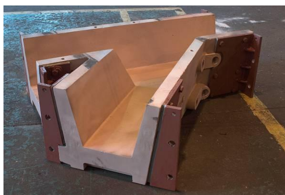
Figure 11: BCL launder - trial assembly
