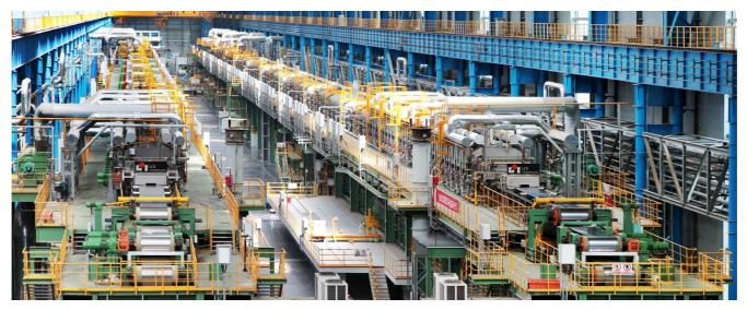
*Tenova LOI Thermprocess,* Two of a total of seven previously delivered heat treatment plants for electrical steel to Shougang.
