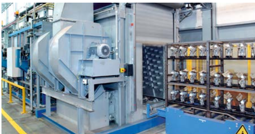
▲ Air quenching chamber for structural components 结构件的气淬室
