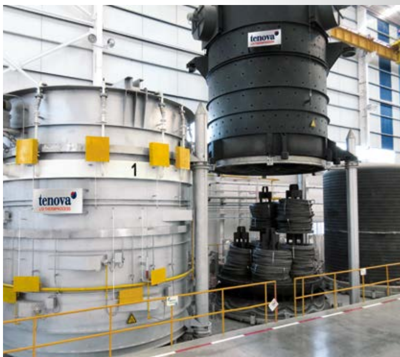
▲ HPH® Bell-type Annealing Plant for CHQ wire
