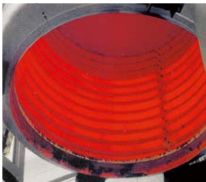
▲ Electrical heating with different zones, thyristor or on/off-controlled
