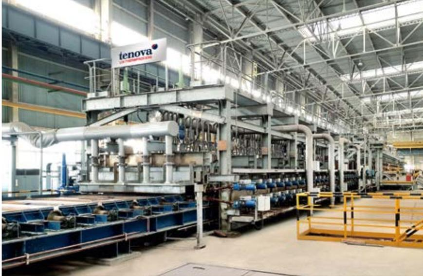
◀ High-throughput continuous quench for heavy plates.
