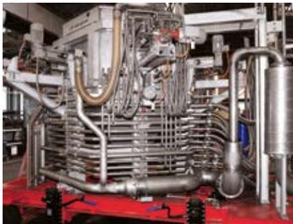
A highly complex quench process with a dedicated system of nozzles spraying water with different flows depending on position and time is essential for ensuring that the forged wheel has a long service life. ▲ ►
