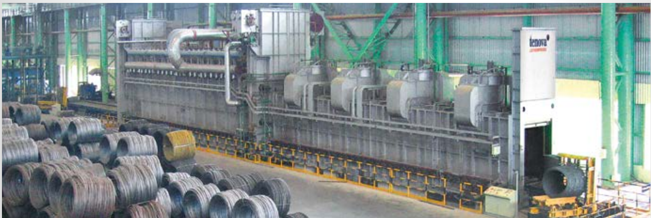
▼ Roller Hearth Furnace for wire coils, type DR 4500
