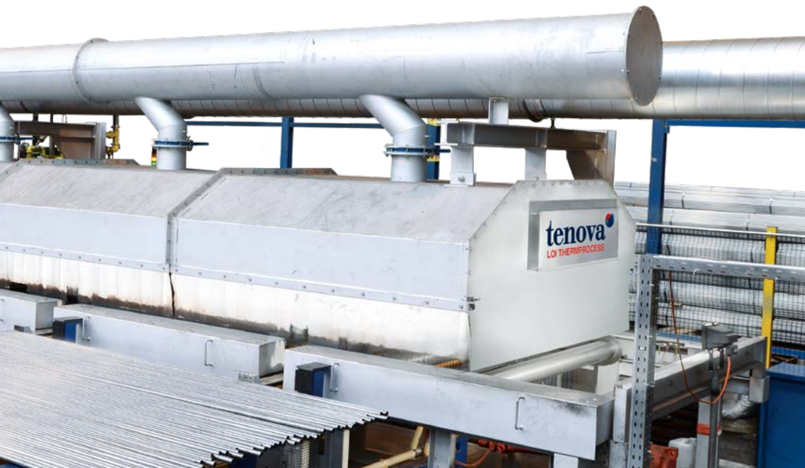
▼ Roller Hearth Furnace for the bright annealing of precision steel tubes
