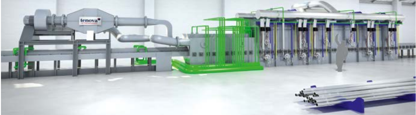
▲ 3-D illustration of a Roller Hearth Furnace for high-alloy steel tubes with hydrogen jet cooling
