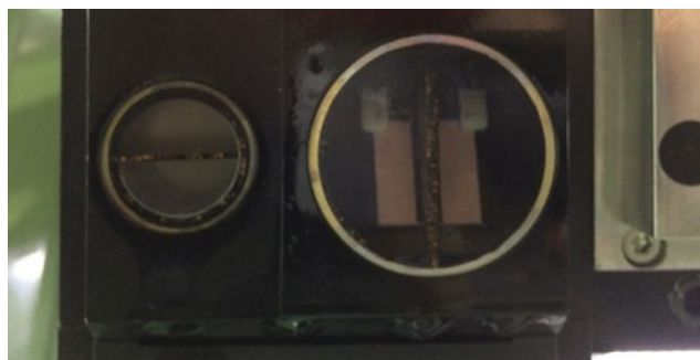
► Left Side is the US (0°) degree probe while on right side the Ultrasound Creeping Wave
