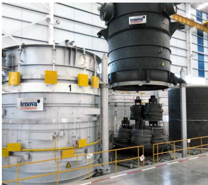
▲ HPH® Bell-type Annealing Plant for CHQ wire
