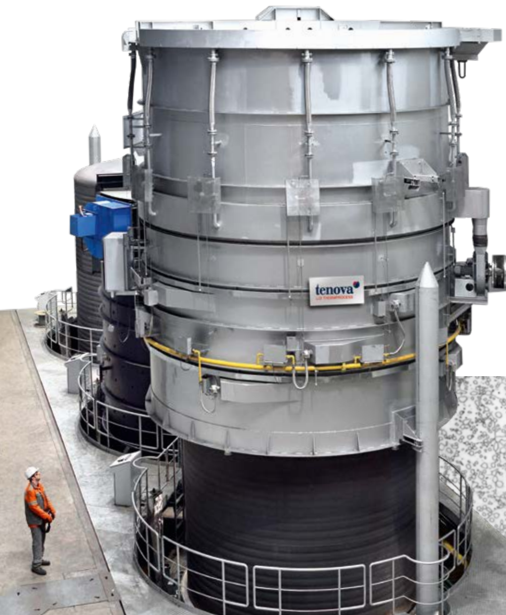
◀ HPH® Heating hood placed over the inner cover with baffle inside
