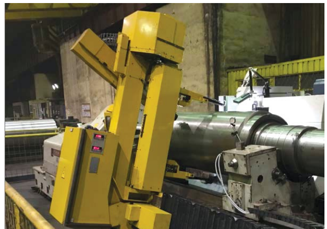
| Replacement Caliper Mounted on Independent Bed
